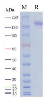
On SDS-PAGE under reducing (R) condition. The gel was stained overnight with Coomassie Blue. The purity of the protein is greater than 95%.
